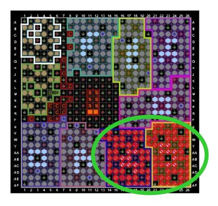
The number of pins available for placement might be reduced when you select additional alternate parts
