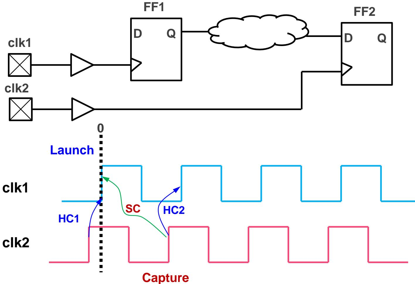
In this example, the default setup and hold analysis returns the preferred requirements and no multicycle exceptions are required
