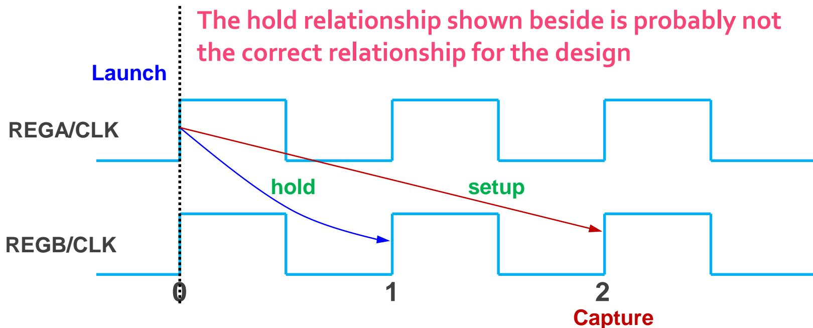
**Hold Check Is Based on Setup Check!**
