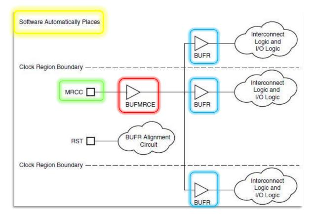
If the divide value in the BUFR is being used, then all BUFR instances must be reset while the BUFMRCE is disabled
