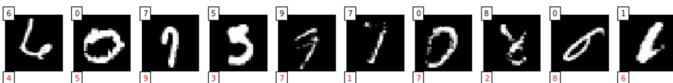
Figure 8.4: Examples of wrong classifications in MNIST dataset. Digits on the upper-left corner are correct labels, and digits on the lower-left corner are predicted labels
